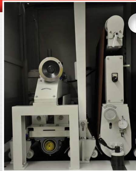
Picture A: Barrel brush head with variable speed and oscillation
