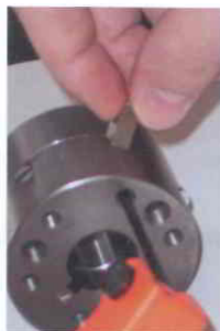
ABOVE: Split Shear Roll assembly on Male Button Lock can be resharpened and features multiple keyways for new shear points.
