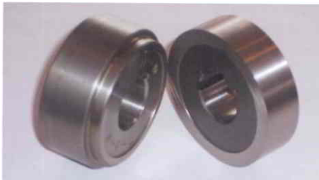
ABOVE: Split Shear Roll assembly on Male Button Lock can be resharpened and features multiple keyways for new shear points.
