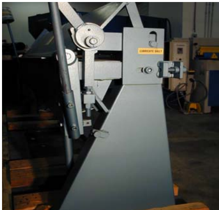
When the shipping skids have been removed, the new brake should be bolted to the floor before operating.
