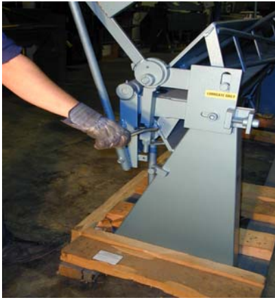
For clamping adjustment, adjust by means of clamping handle adjusting nuts as shown here.
