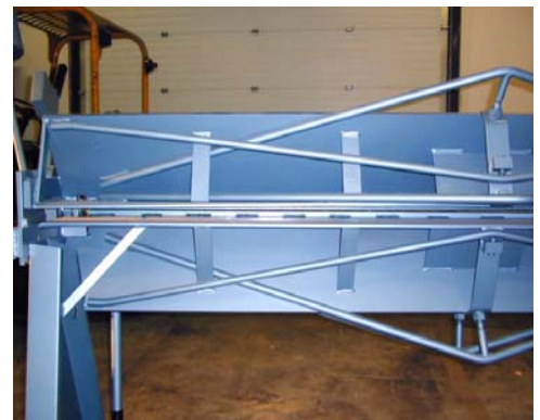
To correct a clicking or snapping bending leaf, it is necessary to adjust the bending leaf center truss nut, and release the center bed adjusting nut.
