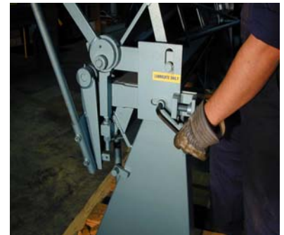
For adjustment of top leaf of brake, slot casting bolt is released as shown here.
