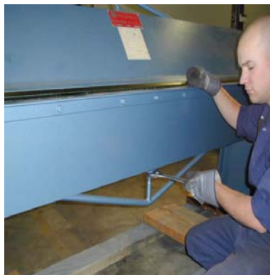
To correct clicking or snapping bending leaf, tighten the truss rod bolt on the bottom of the bending leaf.
