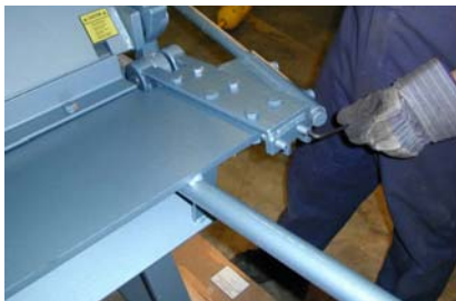
To realign the bending leaf, release the bolts that fasten the hinge to the bending leaf plate, as shown.
