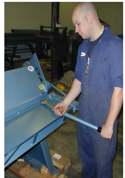
Shown here angle iron being removed. With angle bar removed brake capacity is reduced by four gauges.
