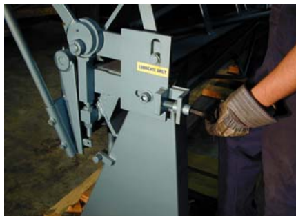
For further adjustment of top leaf of brake, after releasing slot casting bolt, set screws as shown here, are adjusted to push or pull to desired setting.
