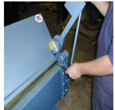
Showing how hand brake capacity is established with the bending leaf angle bar in the high position
