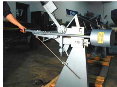
To obtain duplicate bends, position the adjustable stop gauge on the rod, as shown, to the desired setting
