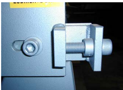
To adjust the leveling, be sure that the bed adjustment saddle and top adjustment screw collar are locked into position so that the adjustment screw cannot move back and forth.
